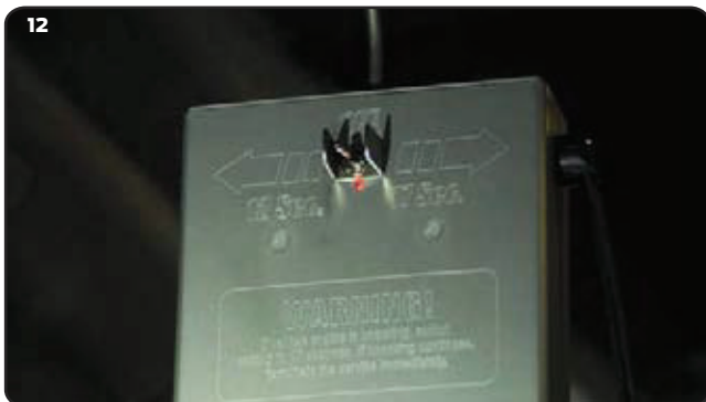
11 & 12 The directional toggle and indicator lights show when and for how long the cleaner is flowing.
