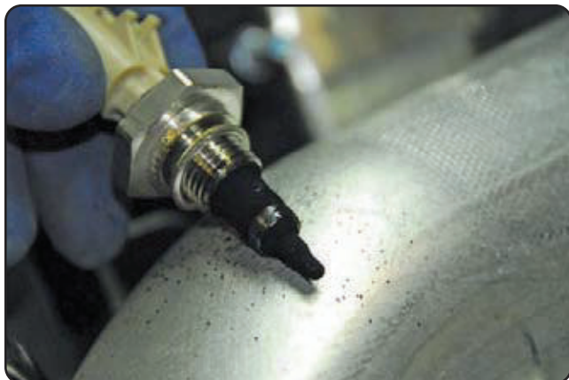
3 Carbon deposits were clearly obvious on this sensor. Buildup of this contaminant robs performance and increases emissions, among other problems.
