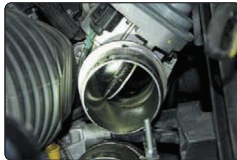
4 After disconnecting the intake hose, additional carbon was also evident.
