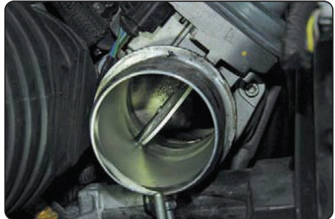
16 The throttle body has noticeably less black carbon after cleaning.
