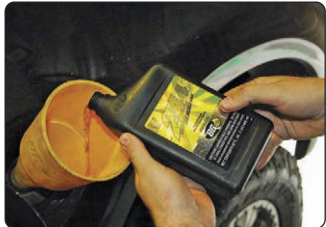
13 BG 244 is a separate cleaner added directly to the fuel tank.
