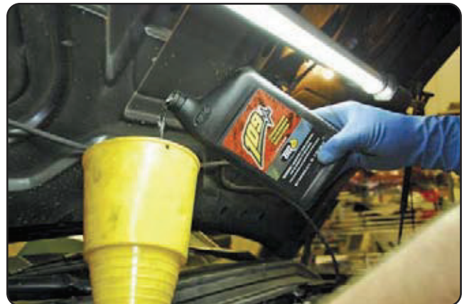
14 BG 109 Compression Performance Restoration is a blend of cleaners designed to soften, emulsify and dissolve fuel gums that clog rings. Removal of these deposits should increase compression and also lower tailpipe emissions, eliminate oil consumption associated with buildup, and improve overall power and economy.
