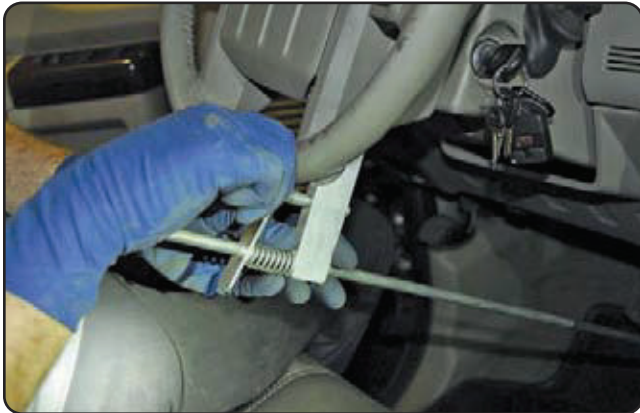
10 A throttle-pedal post maintains engine rpm slightly above idle for about 45 minutes while the cleaner runs through the induction system.
