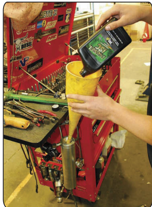
5 Cleaning out the carbon begins with adding Diesel ISC (Induction System Cleaner) to the reservoir in the Diesel Induction Service Set.
