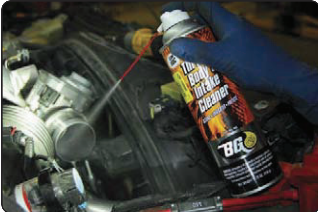
15 Additional deposits were removed by spraying on Throttle Body and Intake Cleaner.
