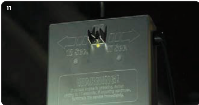
11 & 12 The directional toggle and indicator lights show when and for how long the cleaner is flowing.
