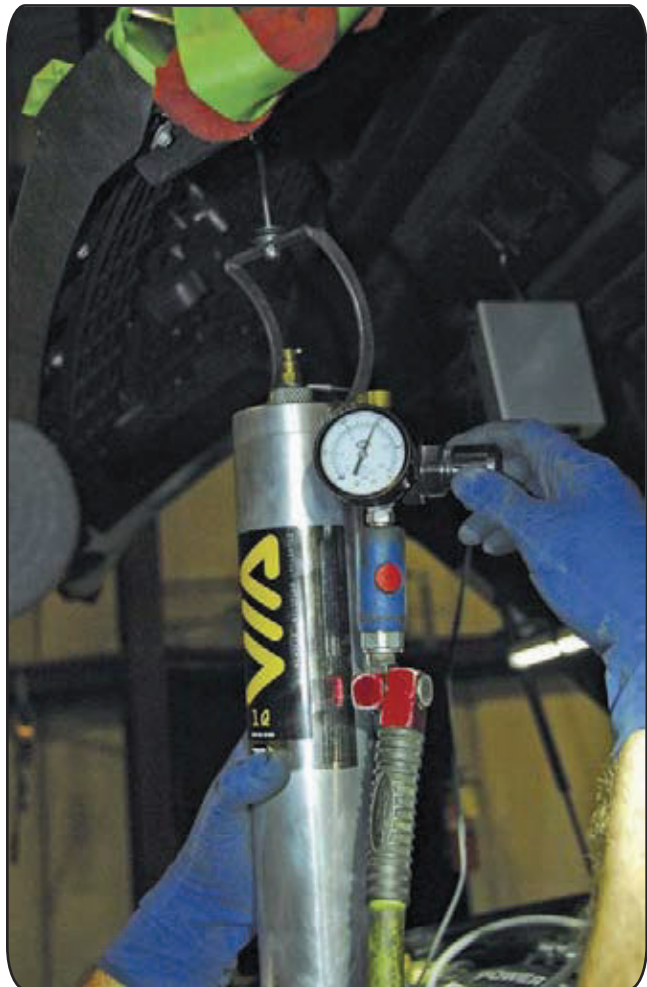
9 The cleaners flow through the intake at a designated pressure for a specified amount of time.
