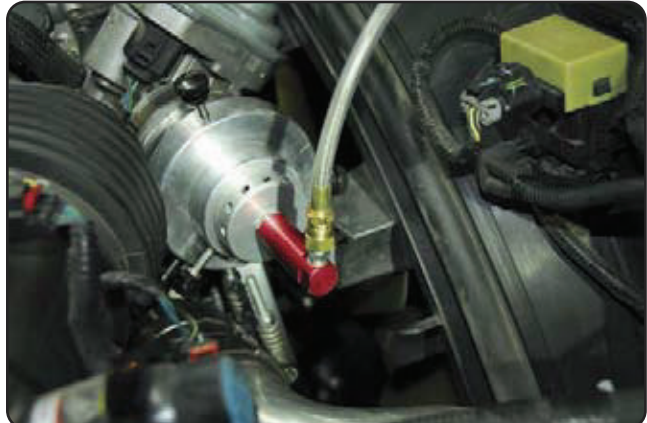
8 The throttle body is capped off with a special cover featuring a hose fitting that's supplied with the Diesel Induction Service Set.
