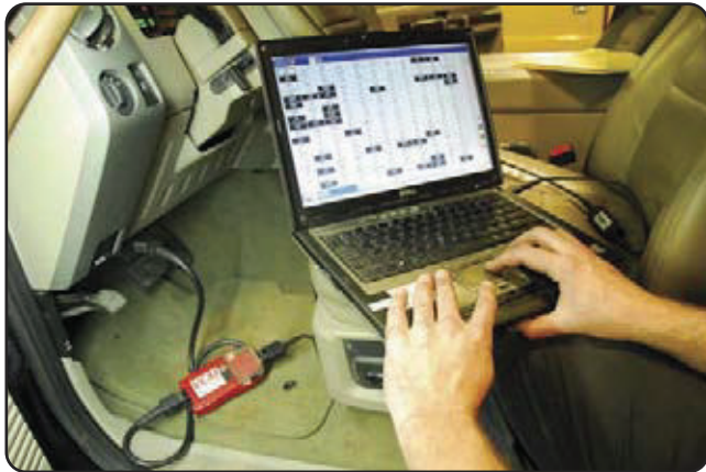
2 Before and after readouts from the engine computer indicated that both the mass fuel and engine load were significantly reduced from "dirty" to "clean" levels.
